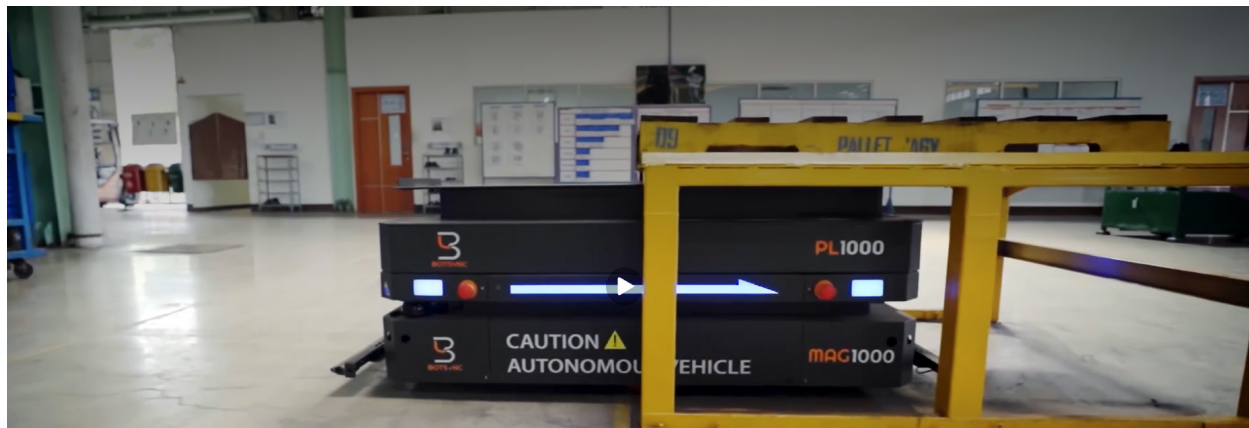
Botsync's MAG1000 Lifter AMR moves heavy parts across the PT Tri Centrum Fortuna factory floor
