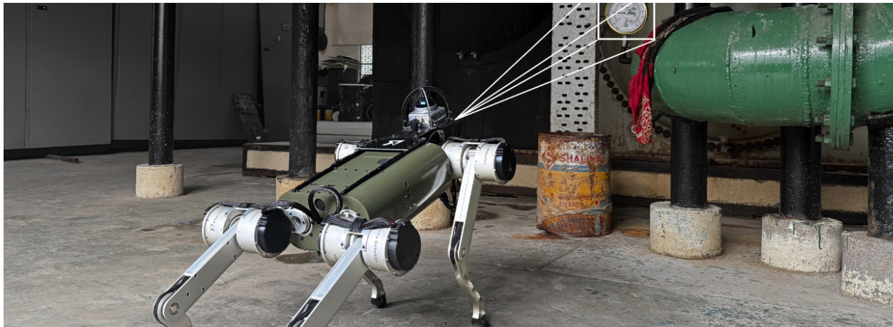
Svan M2 performing autonomous visual inspection of analog gauges in an industrial facility.
