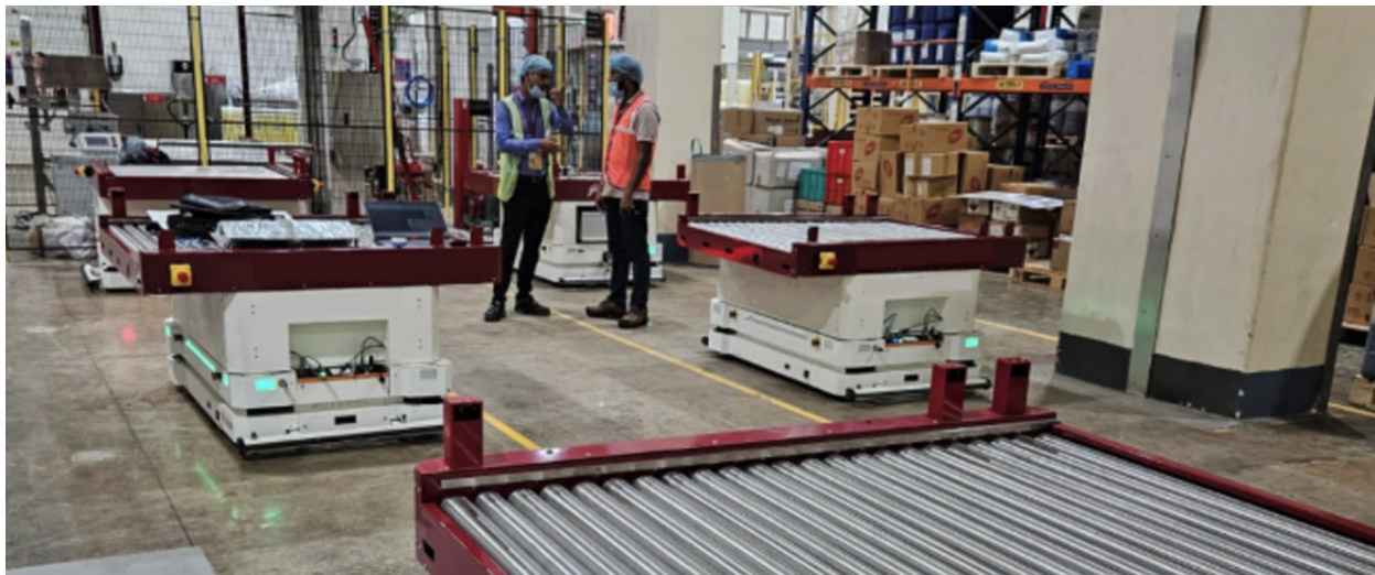
MAG AMR integrated with conveyor and strapping systems for automated pallet transfer
