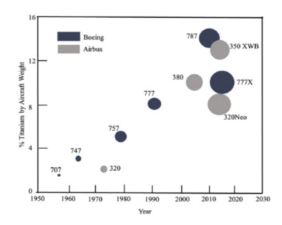
Fig. 2.1.1: Usage of Ti-alloys in commercial airplanes [Sankaran 2017]
