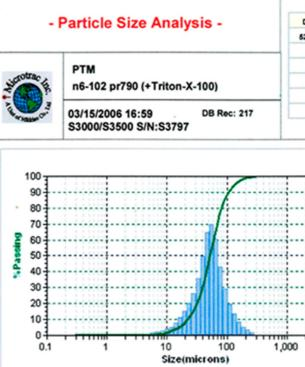
At the client's request, other requirements are possible for the chemical and granulometric compositions. In particular, for plasma coating deposition, a titanium product is produced with fractions of 40-100, 40-140, and 63-160 microns.
