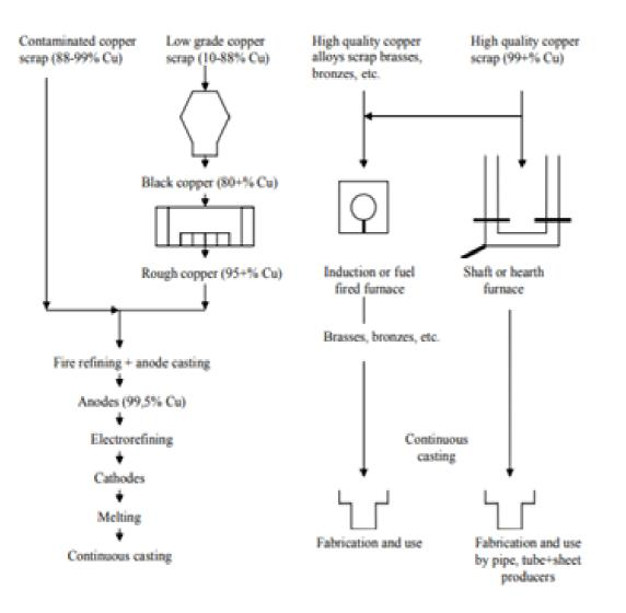
Figure 21: Flow sheet of processes for the recovery of copper and copper alloys from scrap. Low grade scrap is usually smelted in shaft furnaces but also in other furnaces, e.g. electric.
