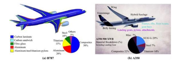
Figure 6.8.3 Distribution map of composites in (a) B787 and 797 (b) A350-900 XWB [16]
