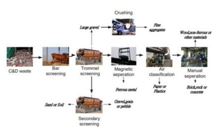
Figure 18: Process flow for C&D waste recycling in Taiwan
