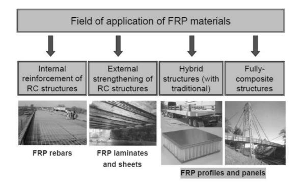
Figure 2.8.2. The significant fields of FRP composites applications [15]
