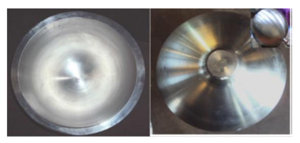
Fig. 2.5.1: Forged & Machined Hemisphere (inset: pressure vessel made out of hemispheres) [Gupta 2015].
