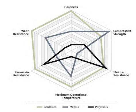
Figure 3.1.1 Properties of advanced ceramics vis a vis metals and polymers
