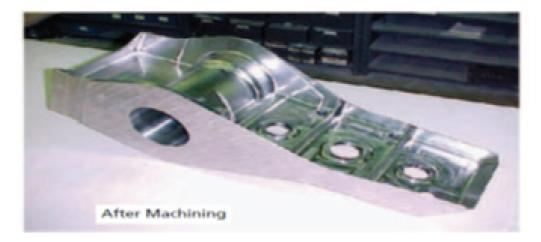
Fig. 2.5.3: Titanium Laser Deposited Rib Section [Campbell 2006]
